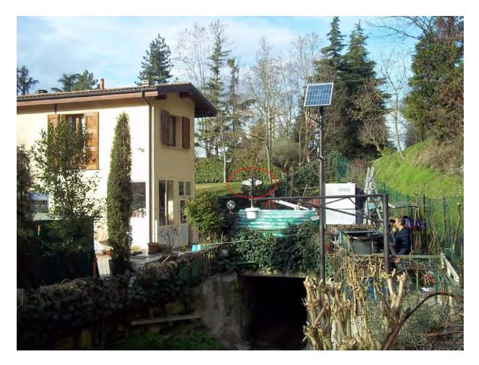
The existing station on the Ravone culvert entry; the new webcam (red circle) is located in correspondence of the hydrometer
