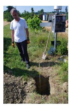
The soil moisture probes placement in correspondence the Mount Paderno CAE weather station
